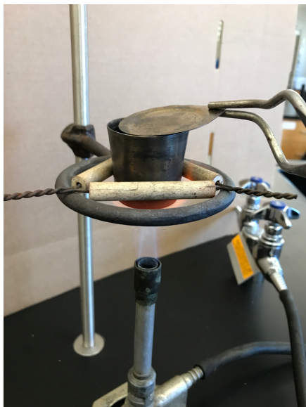
Figure 1: Crucible setup for heating on a Bunsen burner.
